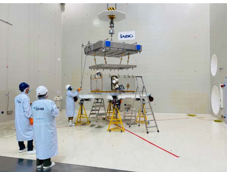
The EnMAP instrument is being lifted out of IABG's sound laboratory by an overhead crane
