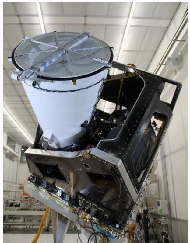
The telescope assembly is an instrument of the MTG weather satellite of the "imager" type, which – to put it simply – is a complex mirror system
