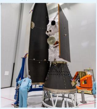
Encapsulation of the satellite in the payload fairing
