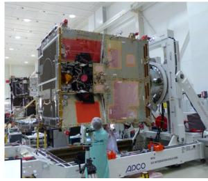
First imager satellite platform in the clean room of OHB System in Bremen just prior to delivery  $\,$
