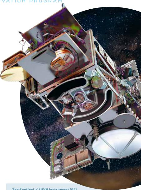
The Sentinel-4/UVN instrument (S4) is part of ESA's Copernicus program. It is mounted as an additional payload on the MTG-S satellites. In the case of Sentinel-4,
