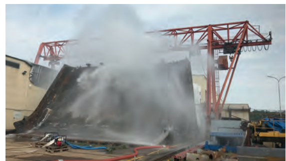
Deflector testing a water cooling subsystem at a plant in the Czech Republic
