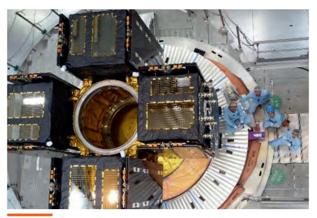
Four Galilean Satellites at final assembly on top of the launch vehicle
