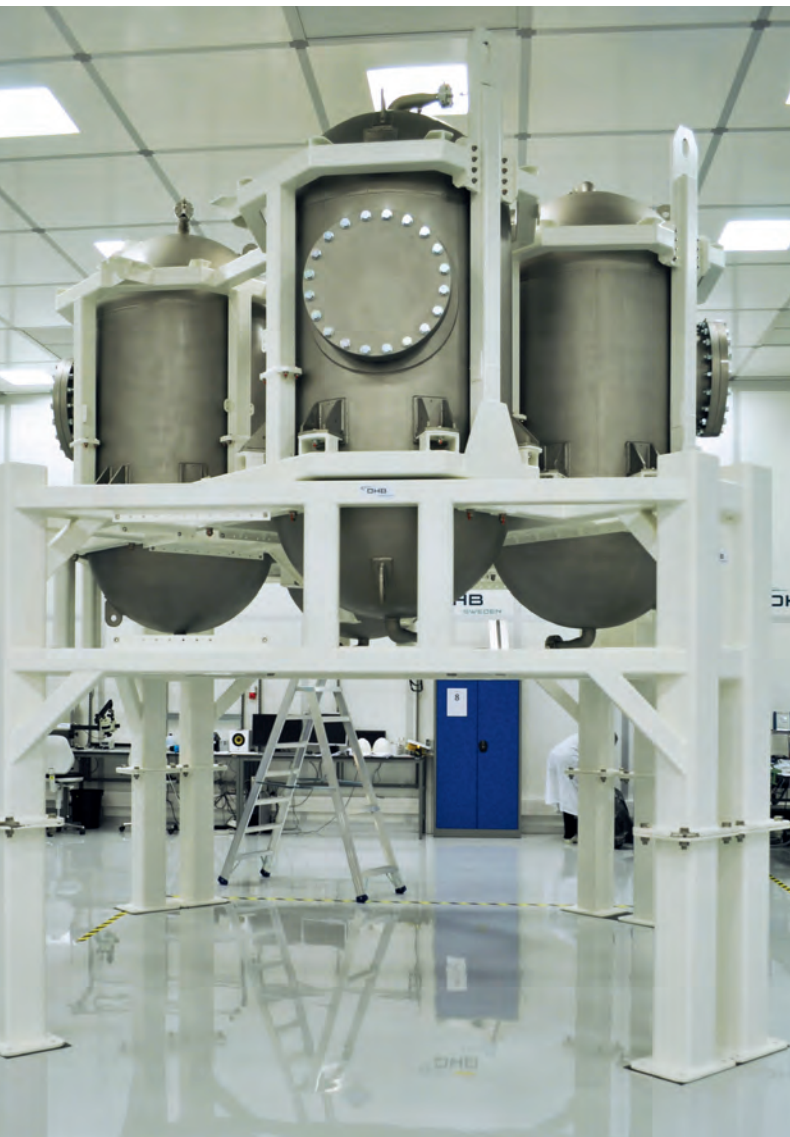
The PQM for the Orion European Service Module in OHB Sweden's clean-room
