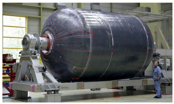
Booster made from carbon fibre-reinforced plastic (CRP) in a partnership between DLR and MT Aerospace
