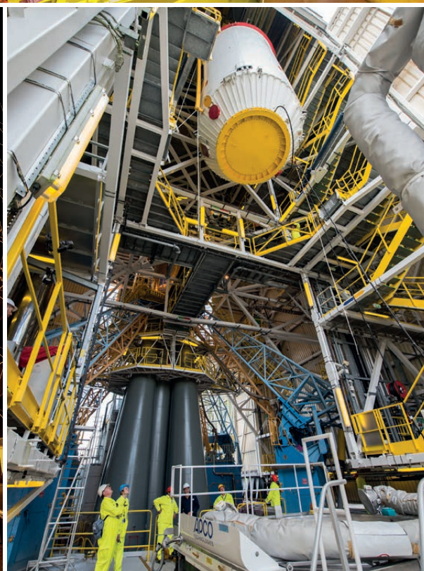
top: Galileo FOC* navigation satellites 9-10 are positioned inside the Soyuz fairing; left: Galileo* liftoff; right: Galileos* hoisted atop Soyuz
