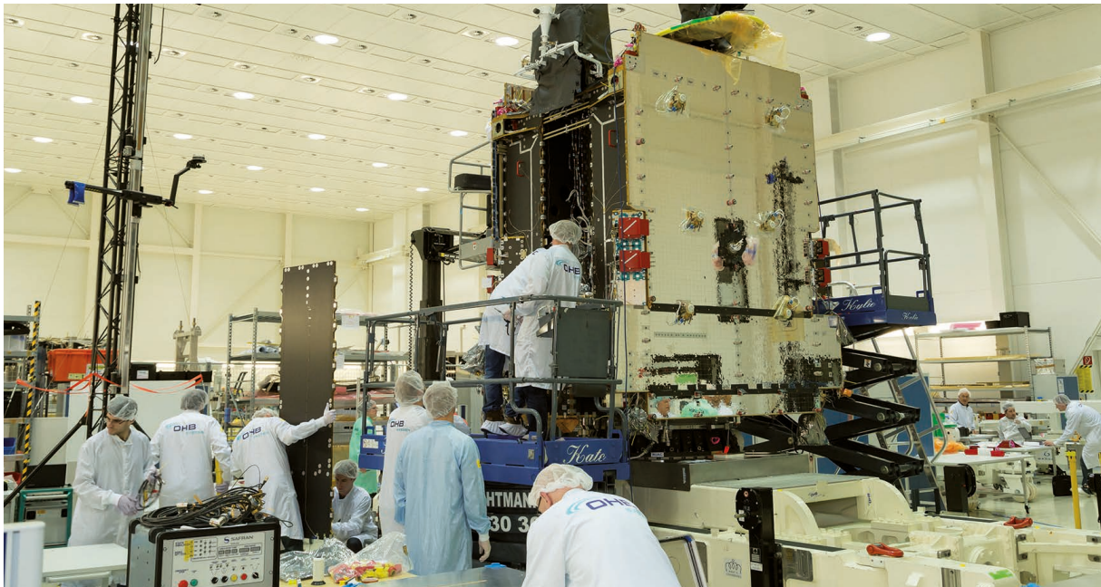
“Hispasat Advanced Generation 1” fully integrated in the OHB clean-room facilities
