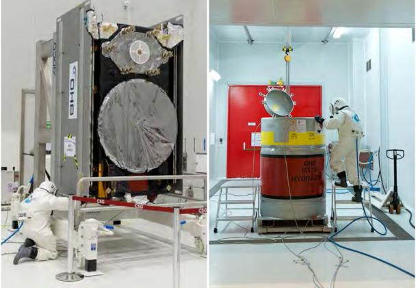
Fueling the tanks of the satellites as final preparation for launch in Kourou, French-Guyana
