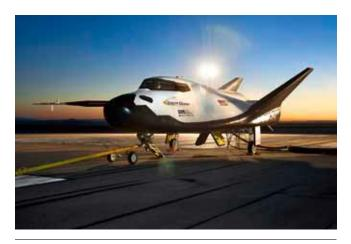
SNC's Dream Chaser® 1:1 prototype for in-flight testing
