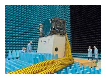
Galileo FOC FM1 during preparations for the PIM test
