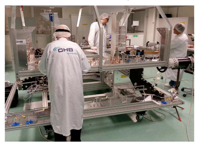
Fixing and testing of the position control system for the SmallGEO satellite at OHB Sweden
