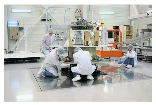
Preparation of the LARES system for the integration in the Vega launcher
