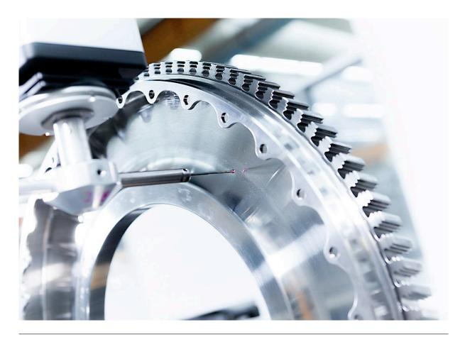
Computer-controlled measurement of an engine disk
