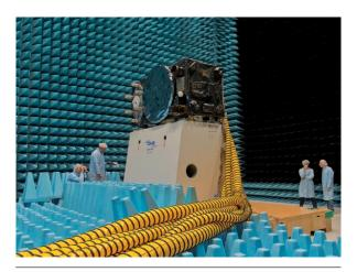
Galileo\* Full Operational Capability (FOC) satellite first flight model, FM1, being prepared for passive intermodulation testing' within the Maxwell electromagnetic test facility inside the ESTEC Test Centre at the end of August 2013.
