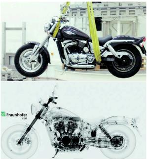
First light tested on a motor cycle using the new X-ray technology
