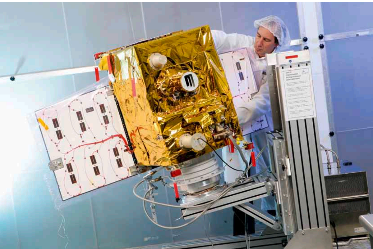
Top: launch of a Soyuz carrying TET-1 on board; bottom: TET-1 being integrated at Kayser-Threde's clean-room facilities
