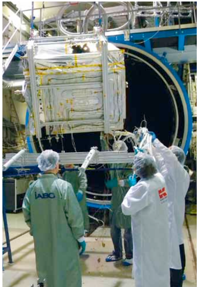
EnMAP before the thermal vacuum test at IAGB mbH in Munich
