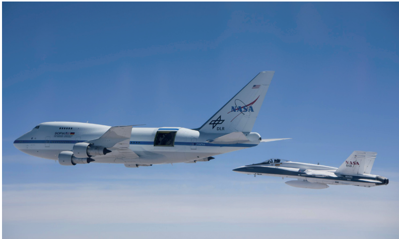
Unique SOFIA telescope fitted to the tail of a modified Boeing 747SP
