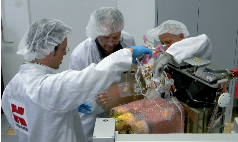
Integration of the TET satellite (platform with payload) at Kayser-Threde's clean room.
