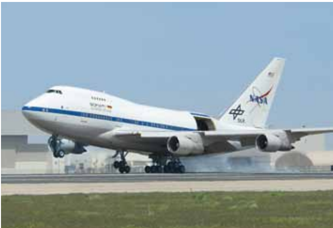
SOFIA: NASA Boeing 747 with an open hatch, behind which the telescope is located.
