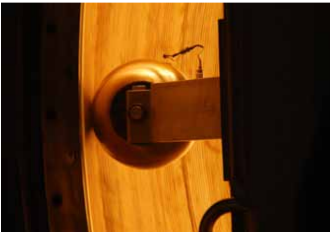
Friction-stir-welding of a tank dome at MT Aerospace in Augsburg
