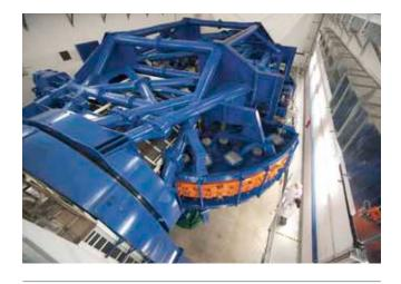
The Heidelberg Ion Radiation Therapy Center HIT. MT Aerospace provided the world's first rotating gantry.
