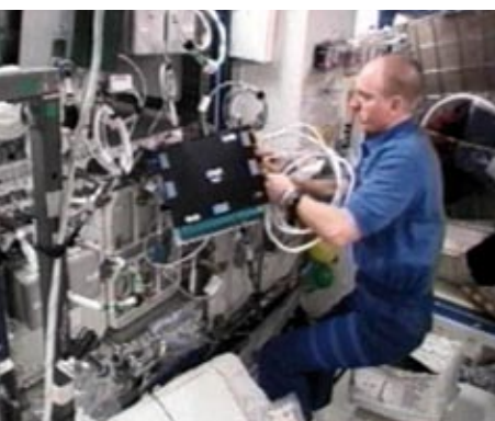
NASA astronaut Clayton C. Anderson installing the gas analyzer on board the ISS
