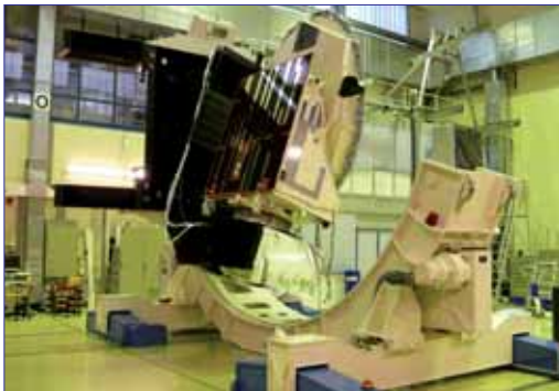
Environmental testing of the SAR-Lupe FM 2 reconnaissance satellite at IABG in Ottobrunn
