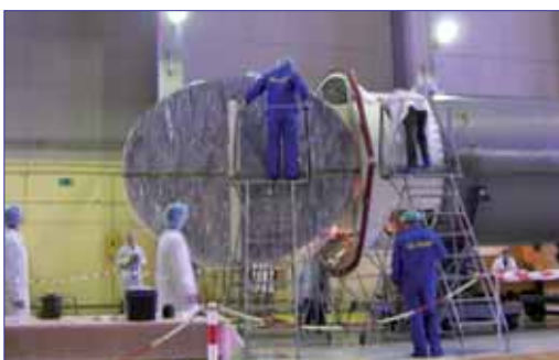
Assembly of the SAR-Lupe FM 2 into the COSMOS 3M launch vehicle in Plesetsk
