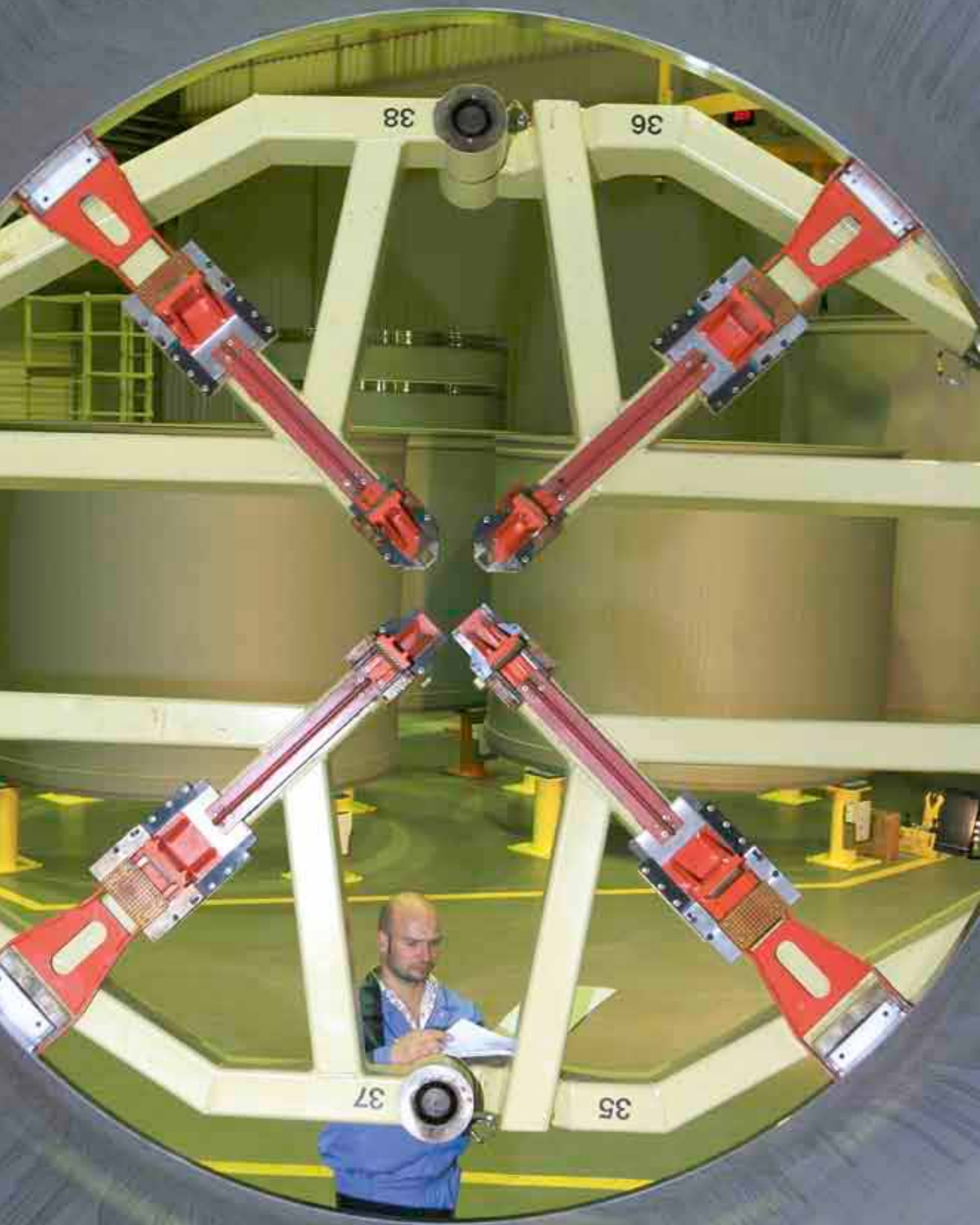
Receiving attention from all sides: a component for the Ariane booster case in the rolover machine.
