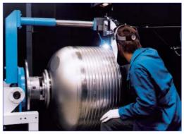
Production of a waste water tank for the Airbus A340
