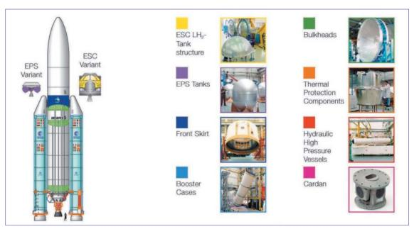
MT Aerospace: Components developed for the Ariane 5
