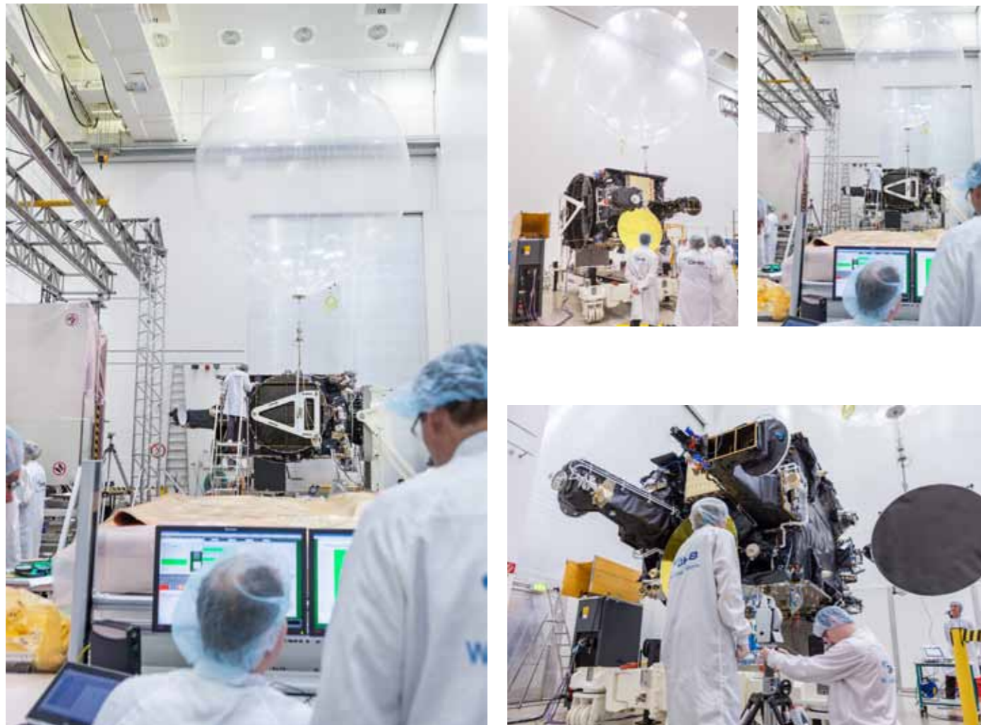
Test campaign (antenna alignment) at test house IABG in January 2016.
