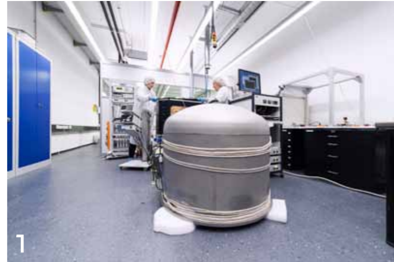
1 Thermal/vacuum laboratory under ISO8 conditions. The thermal conditions prevailing in space to which components and systems are exposed over a specified duration can be simulated in the chambers.
